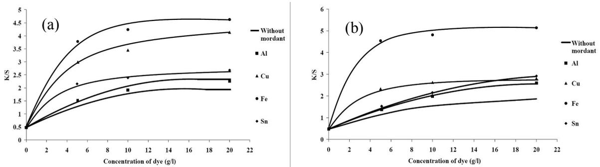
**Figure 15** Effect of dye concentrations on  $K/S$  values of wool fabric dyed with 10 g/l mordants by simultaneous mordanting and using (a) pad-batch technique (b) pad-dry technique
