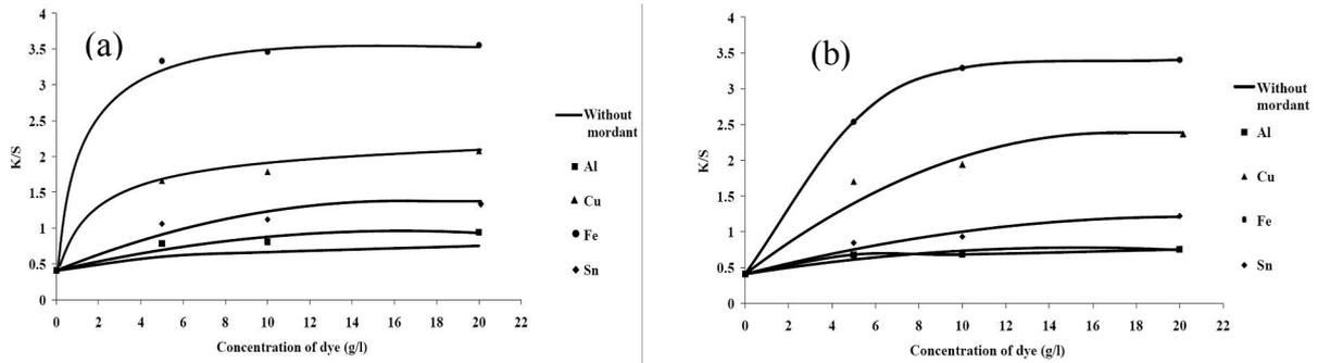
**Figure 13** Effect of dye concentrations on  $K/S$  values of silk fabric dyed with 10 g/l mordants by post-mordanting and using (a) pad-batch technique (b) pad-dry technique
