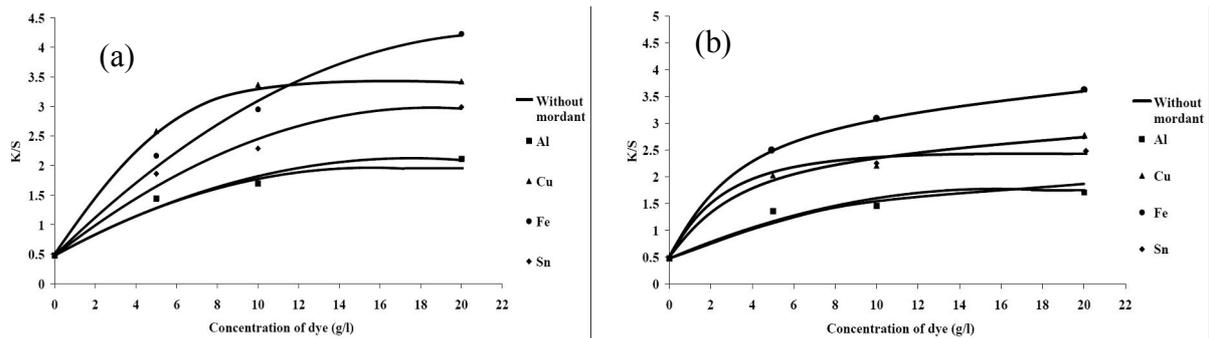
**Figure 14** Effect of dye concentrations on  $K/S$  values of wool fabric dyed with 10 g/l mordants by pre-mordanting and using (a) pad-batch technique (b) pad-dry technique
