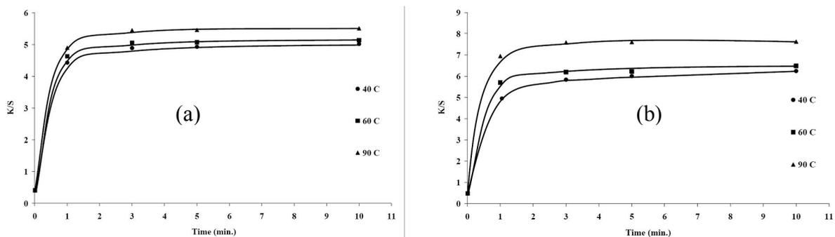
**Figure 19** Effect of drying time and temperature of pad-dry technique on the colour strength ( $K/S$  values) of (a) silk fabric and (b) wool fabric dyed with 20 g/l eucalyptus leaf extract and using 20 g/l ferrous sulfate by using simultaneous mordanting
