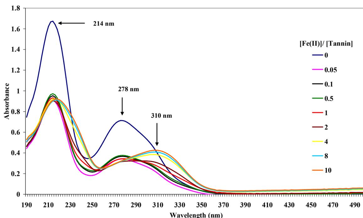
**Figure 5** Absorption spectra of tannin ( $1 \times 10^{-5}$  Molar) in aqueous solution in the absence and in the presence of Fe (II) (0-100 micro molar)
