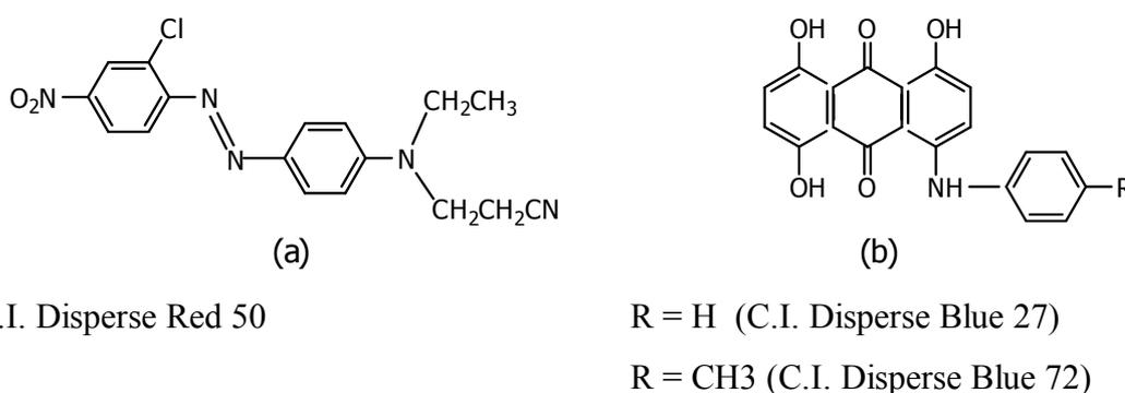
**Figure 2** Chemical constitution of typical disperse dyes. (a) Azo dye and (b) anthraquinone dyes
