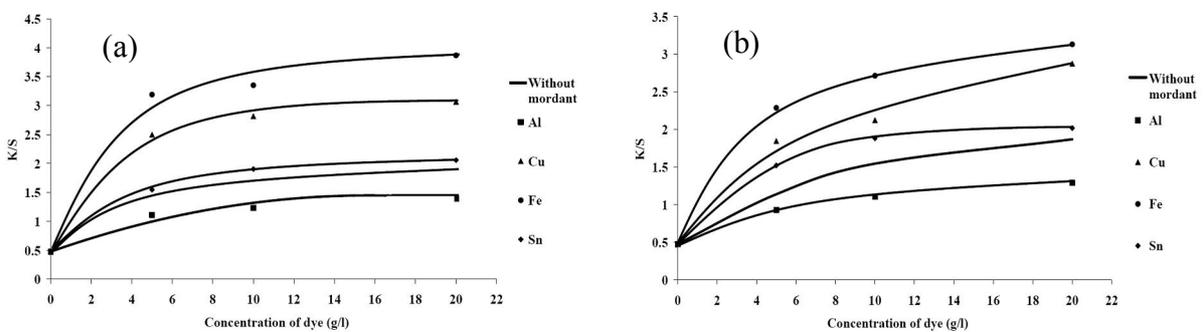
**Figure 16** Effect of dye concentrations on  $K/S$  values of wool fabric dyed with 10 g/l mordants by post-mordanting and using (a) pad-batch technique (b) pad-dry technique
