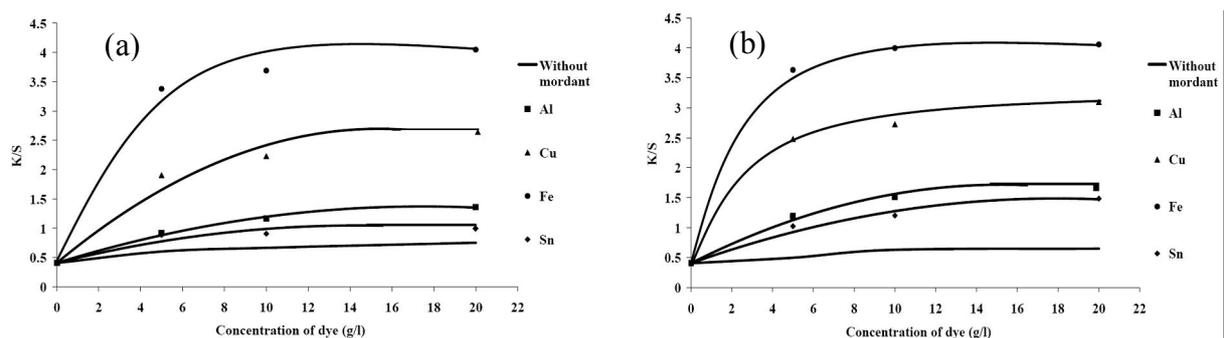
**Figure 12** Effect of dye concentrations on  $K/S$  values of silk fabric dyed with 10 g/l mordants by simultaneous mordanting and using (a) pad-batch technique (b) pad-dry technique
