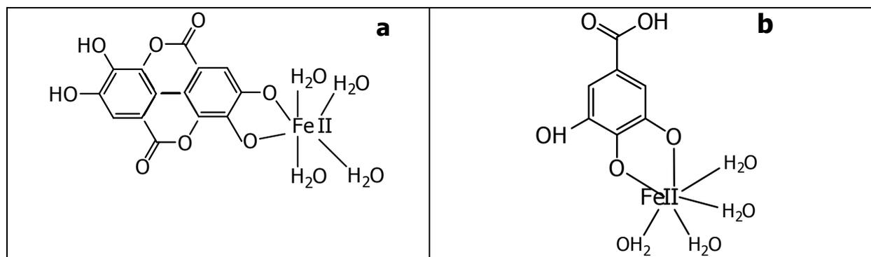
**Figure 8** Proposed the structure of ferrous-tannins complex (a) 1:1  $[\text{Fe(II)}]:\text{ellagic acid}]$ , and (b) 1:1  $[\text{Fe(II)}]:\text{gallic acid}]$
