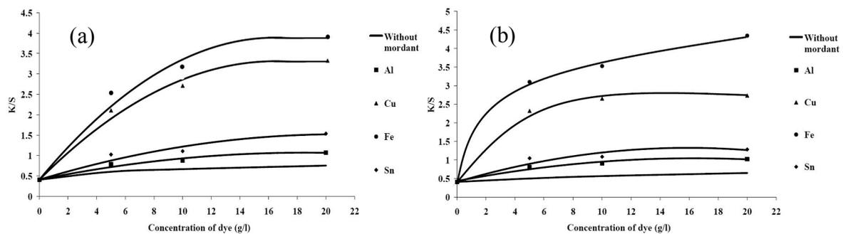
**Figure 11** Effect of dye concentrations on  $K/S$  values of silk fabric dyed with 10 g/l mordants by pre-mordanting and using (a) pad-batch technique (b) pad-dry technique
