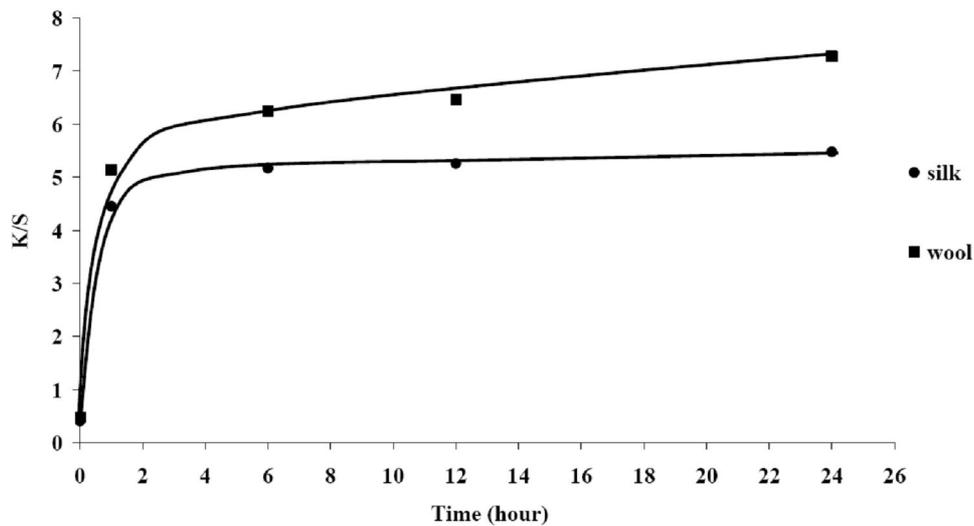
**Figure 20** Effect of batching time of pad-batch technique on the colour strength ( $K/S$  values) of silk and wool fabric dyed with 20 g/l eucalyptus leaf extract and using 20 g/l ferrous sulfate by using simultaneous mordanting
