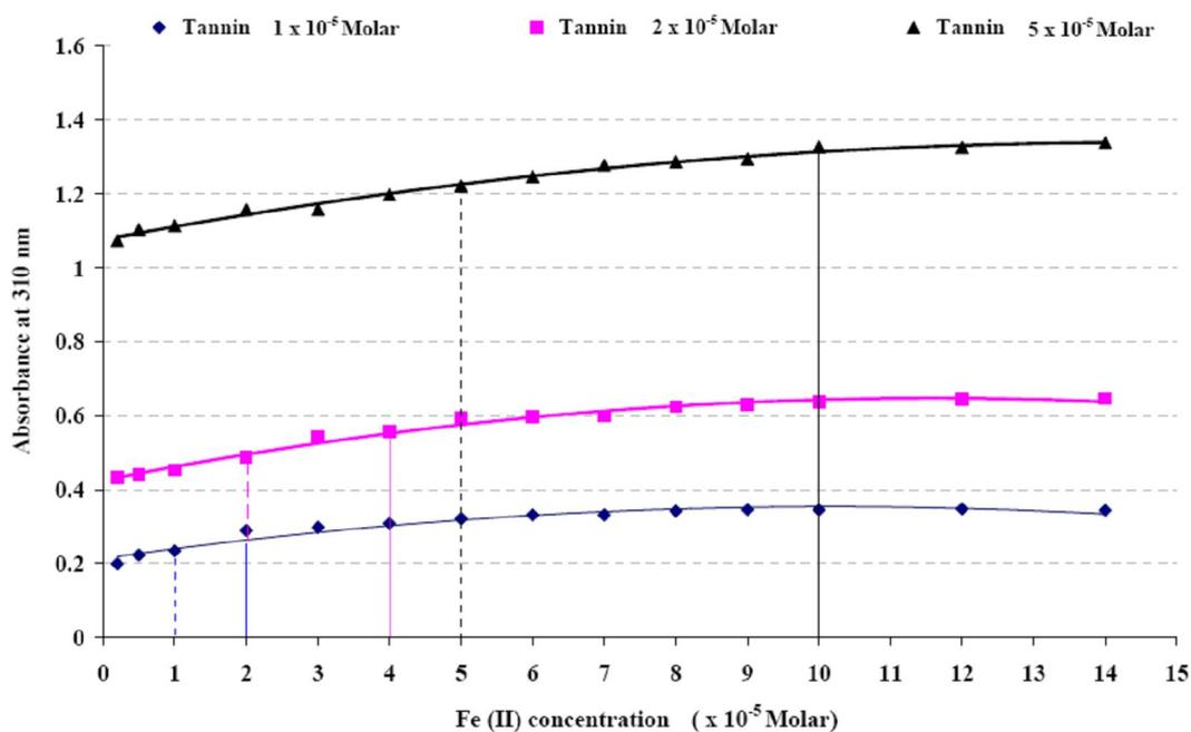
**Figure 7** The effect of Fe (II) concentration on tannin in aqueous solution. Dash line is the [Fe(II)] / [tannin], 1:1. Solid line is the [Fe(II)] / [tannin], 2:1.
