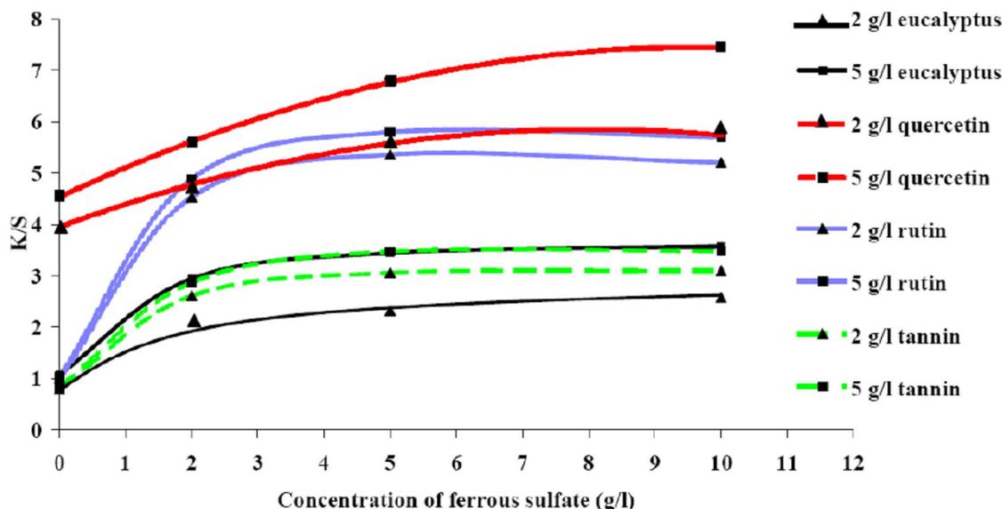
**Figure 21** The  $K/S$  values of dyed wool fabric with eucalyptus leaf extract, quercetin, rutin and tannin dye by varying concentration of dyes and ferrous sulfate
