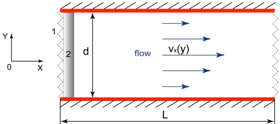
**Figure 8:** The geometry of two-dimensional channel for Poiseuille flow simulation: **1** – periodic boundary conditions, **2** – the imaginary ventilator, **L** is the length and **d** is the width of the channel
