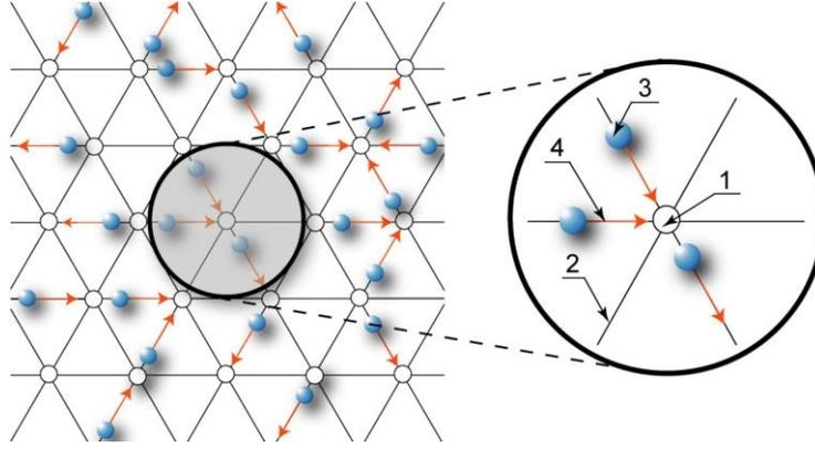
**Figure 2:** Representation of the LGCA model underlaid by the hexagonal Bravais lattice: **1** – the node, i.e. the individual automaton, **2** – the channel, **3** – the moving particle, **4** – the direction of moving [11]
