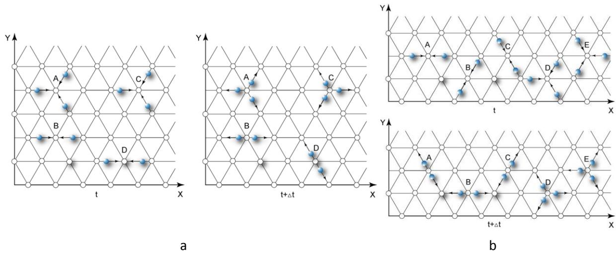
**Figure 3:** Typical two- and three-particle collisions (a) and effective collisions (b) in the FHP-1 LGCA model [11]
