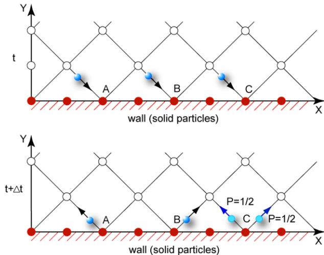
**Figure 5:** Various reflective boundary conditions: **A** - bounce-back reflection, **B** - specular reflection, **C** - diffusive reflection [11]
