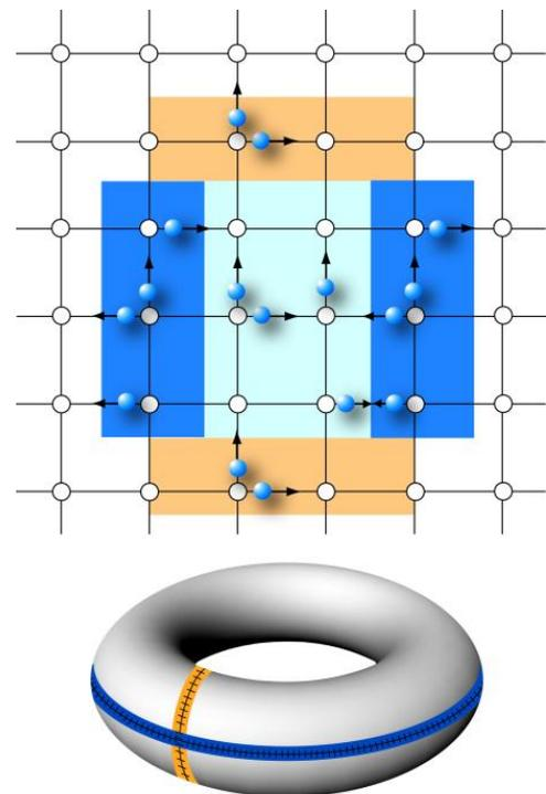
**Figure 4:** The principle of periodic boundary conditions for two-dimensional square LGCA (HPP model) [11]
