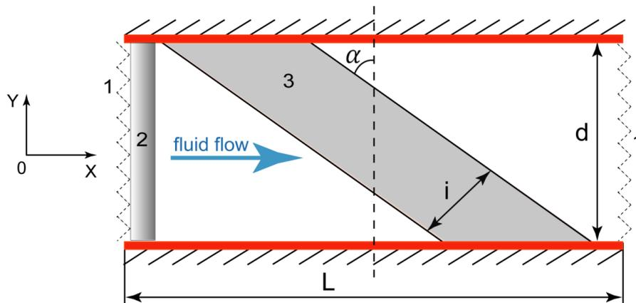
**Figure 11:** The geometry of two-dimensional channel for fluid flow through porous medium simulation:  $L$  is the length and  $d$  is the width of the channel,  $\alpha$  is an inclination angle of the porous medium,  $i$  corresponds to the thickness of the porous medium, 1 – periodic boundary conditions, 2 – the imaginary ventilator created the flow.
